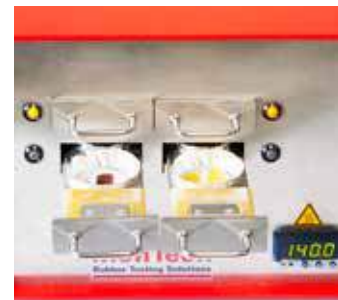
6 - Put drawer back in the oven to start the 30 minute ageing sequence
